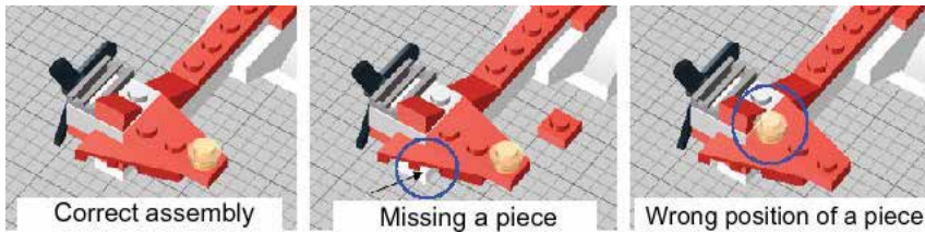
Fig. 12. Examples of a correct assembly, missing a piece and wrong position of a piece.
