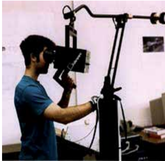
Fig. 2. A binocular omni-orientation monitor (BOOM)
