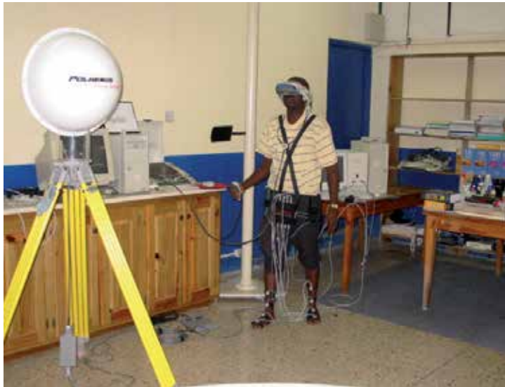
Fig. 3. The Author with the i-glasses PC 3D HR Head Mounted Display and the Polhemus electromagnetic tracker system (Akinladejo, 2005)
