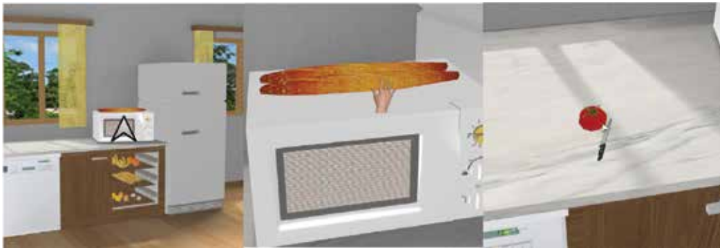
Fig. 9. The three cursor modes: at left an arrow on unreachable objects, in the middle an animation of the hand on reachable objects and, for dragging, the arrow and the held object conveniently scaled, here, the knife.
