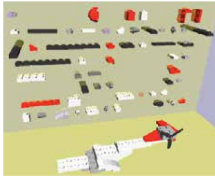
Fig. 5. Virtual assembly scene. Trainees have to grasp the correct piece from the backwall and place it in its correct position in the model.
