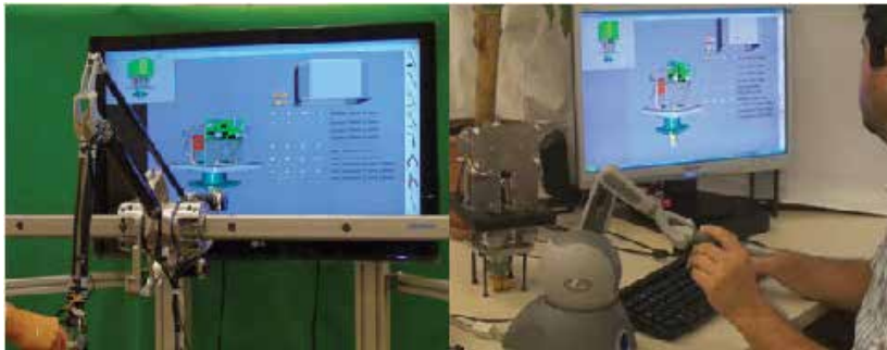
Fig. 4. Multimodal Training System. On the left, the system is configured to use a large workspace haptic device. On the right, the system is configured to use a desktop (small workspace) haptic device.
