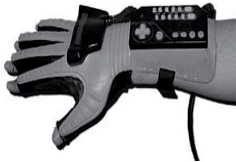
Fig. 5. An instrumented glove (Nintendo power glove)
