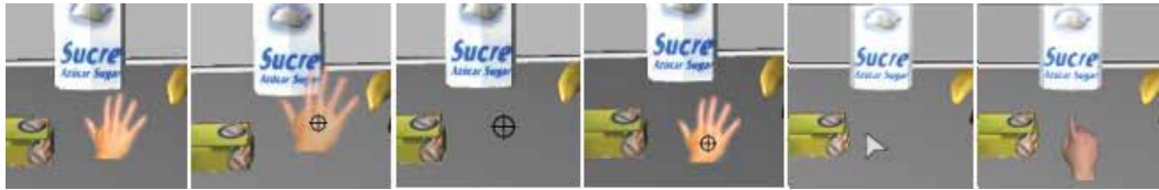
Fig. 1. The six cursors tested. From left to right: opaque hand, transparent hand + spy-hole, spy-hole, opaque hand + spy-hole, arrow, pointing finger
