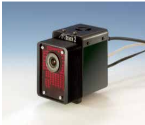
Fig. 4. A.R.T. optical tracking system
