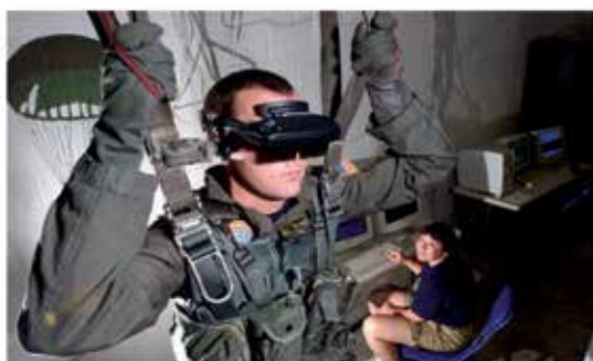
Source description: Hospital Corporal 2nd Class Tim Sudduth, from Vashewick, Wash., demonstrates the Virtual Reality (VR) parachute trainer, while Aviation Survival Equipmentman 1st Class, Jackie Hilles, from Eklund, Penn., controls the program from a computer console. Students wear the VR glasses while suspended in a parachute harness, and then learn to control their movements through a series of computer-simulated scenarios.
