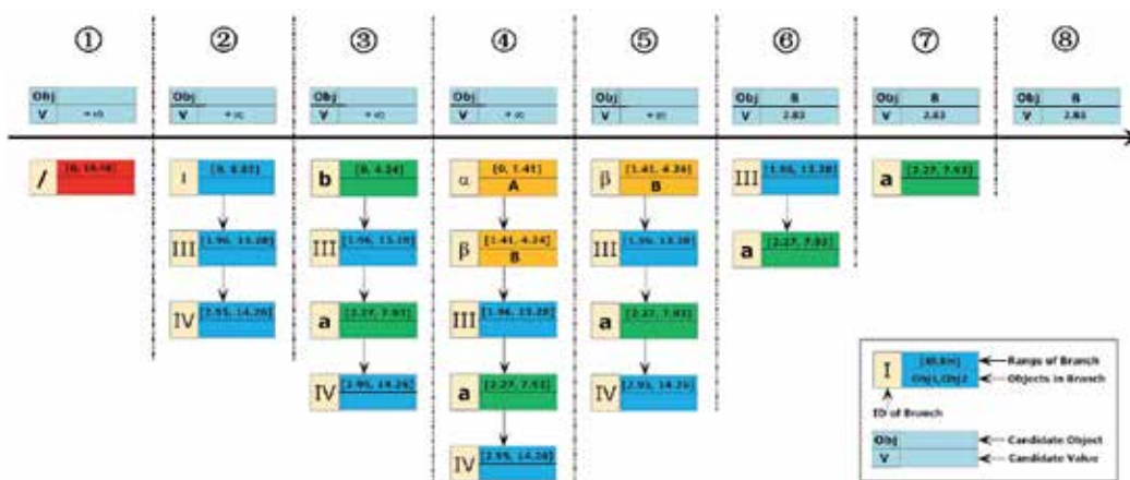
Fig. 14. Scheme for the fast search of the nearest point to a given fixed one.
