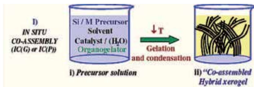
Fig. 3. Strategy for template synthesis of nanotubes mediated by organogelators in-situ coassembly. [Reprinted with permission from (Llusar & Sanchez, 2008), Copyright 2008, American Chemical Society]
