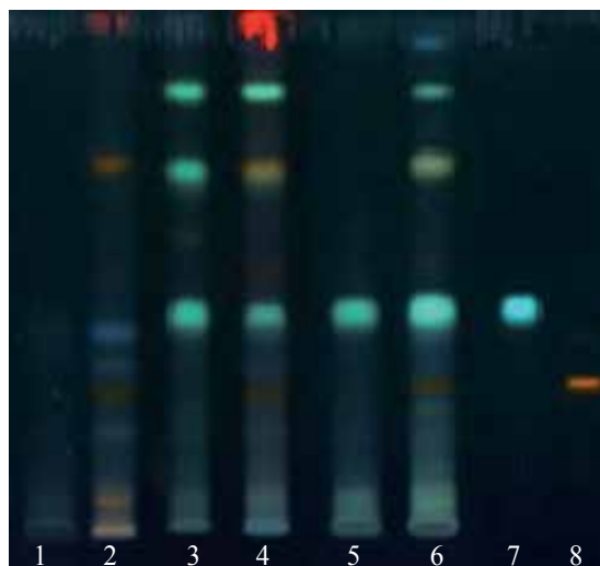
Fig. 3. TLC chromatogram of extracts from A. trifoliatum . Track : 1= root 95% maceration, 2= leaf 95% maceration, 3= root 75% refluxing, 4= leaf 75% refluxing, 5= root decoction, 6= leaf decoction, 7= standard chlorogenic acid, 8= standard quercetin, Stationary phase: silica gel GF254 Solvent system: ethyl acetate: acetic acid : formic acid : water 137: 11: 11: 26 Detection: NP-PEG spraying reagent / UV 366 nm.
