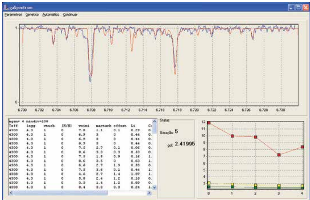
Fig. 7. Main screen of the program GASpectrum after five generations. The upper panel presents the spectra: the blue line represents the observed spectrum and the red line represents the best individual spectrum (adapted from Hetem & Gregorio-Hetem 2009).
