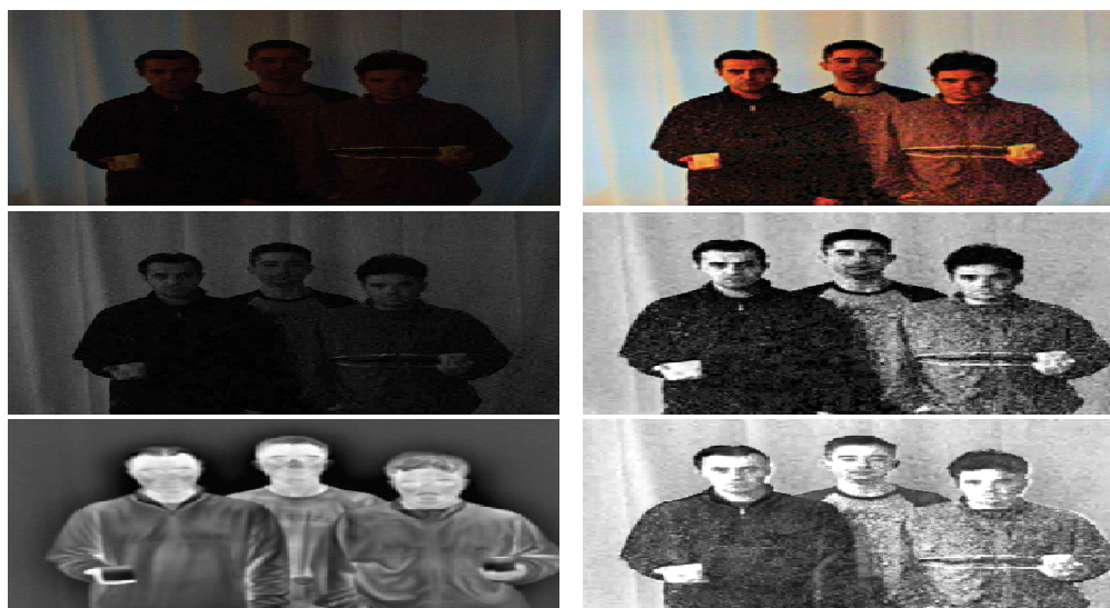
Fig. 6. Fusion Results for Image 1: (top-left-(a)) Original; (top-right-(b)) Enhanced; (middle-left-(c)) Original; (middle-right-(d)) Enhanced; (bottom-left-(e)) IR;(bottom-right-(f)) Fused Images; Graph-Genetic Algorithm result after 100 iterations.
