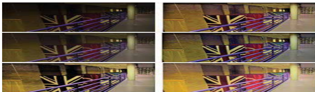
Fig. 2. Comparisons of Enhancement Techniques: (top-left) Original; (top-right) IRME; (middle-left) Gamma correction, g = 1.4 ; (middle-right) MSR; (bottom-left) AINDANE; (bottom-right) ETNUD.
