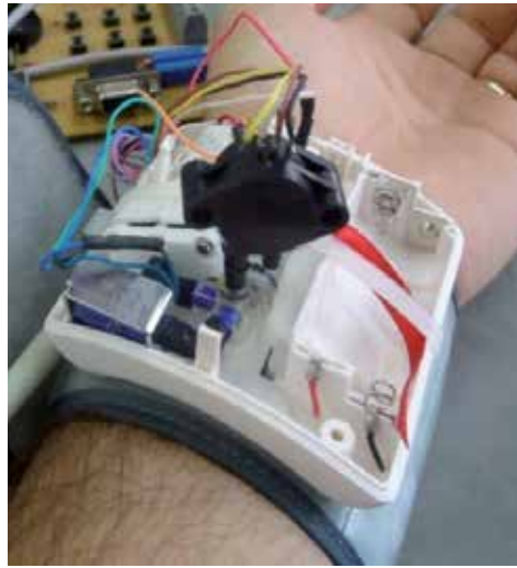
Fig. 11(a). Arterial pressure Prototype for arterial pressure acquisition.
