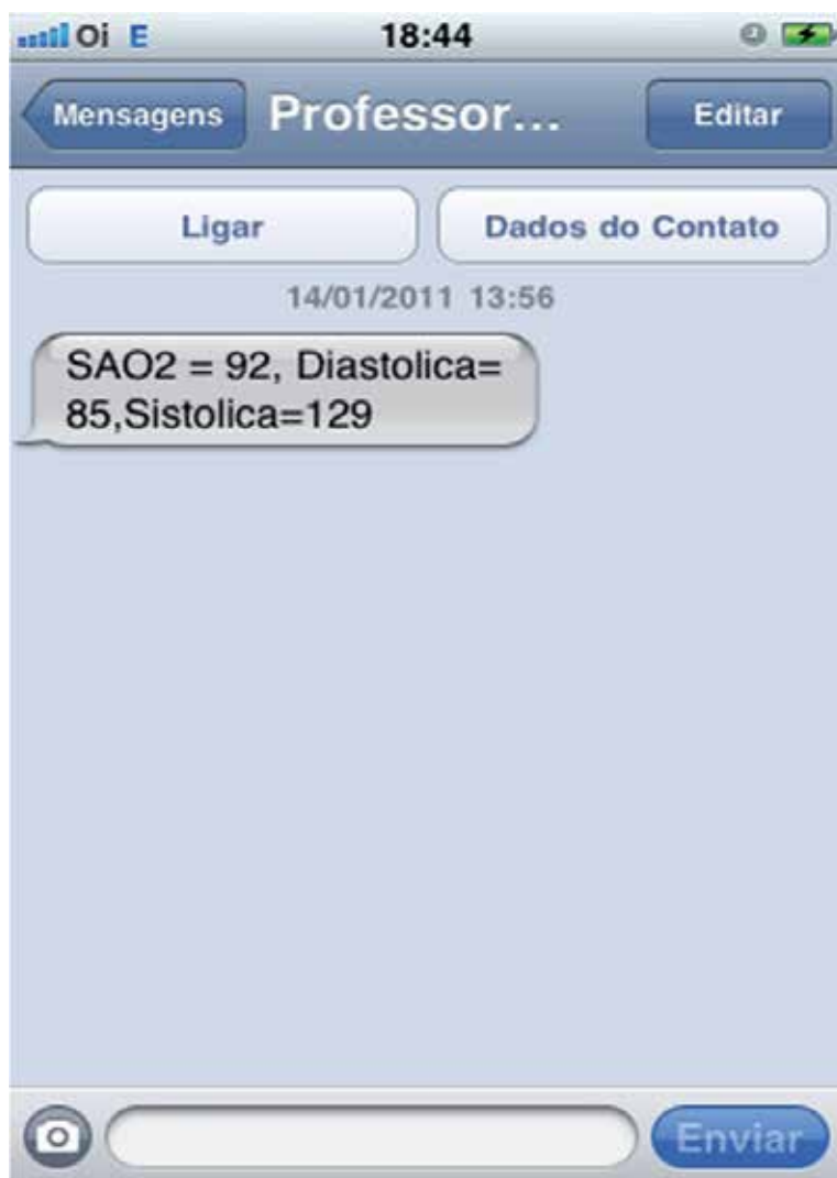
Fig. 13. Oxymeter and blood arterial pressure data sent to a cell phone via GSM communication.
