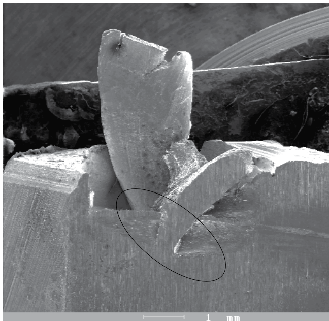
Fig. 19. Cutting zone - Drilling using a helical drill; interaction between the workpiece and tool cutting area
