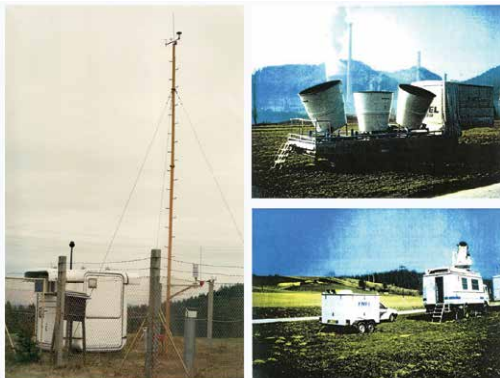
Fig. 7. Pictures of some of equipment used in campaign in spring 1991: environmental automatic measuring station (left), mobile SODAR (right - upper) and DIAL (right -lower)
