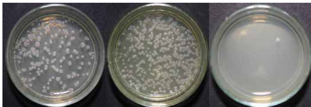
(a) Before treatment. (b) Discharge voltage 1.0 kV. (c) Discharge voltage 1.4 kV.
