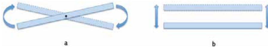
Fig. 1. Methods of whole body vibration stimulation. The figure depicts the two methods of platform oscillation: alternating rotation (a) and vertical oscillation (b).
