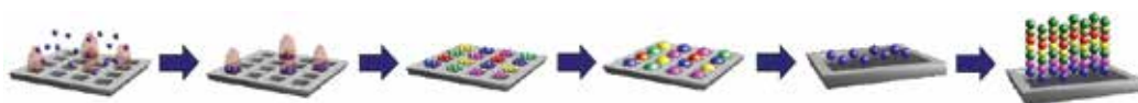
Fig. 1. Left to right: Solid phase peptide synthesis on CMOS chips: Negatively charged micro particles containing amino acids are guided to their synthesis sites by the selectively programmable electric fields of the CMOS chip, particles containing one specific sort of amino acids are deposited, particles containing all sorts of amino acids for the first layer of the peptide array are deposited, heating initiates the coupling of the first layer of amino acids to the surface, remnants of particles and excess amino acids are discarded in chemical washing, repeating this procedure leads to a complete peptide array (From Beyer et al. (2007). Reprinted with permission from AAAS.)
