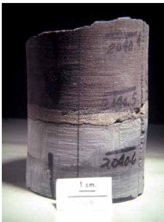
Fig. 4. Black Cleveland Shale above gray Chagrin Shale in an EGSP core from Ohio, with pyrite at the contact (2040.54 ft.). An orientation groove is visible to the right of the depth marks; the vertical line on the front of the core marks north. Photo by Daniel J. Soeder.
