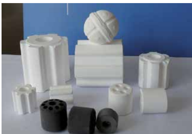
Fig. 5. The novel shapes with high strength of the reforming catalyst and support.
