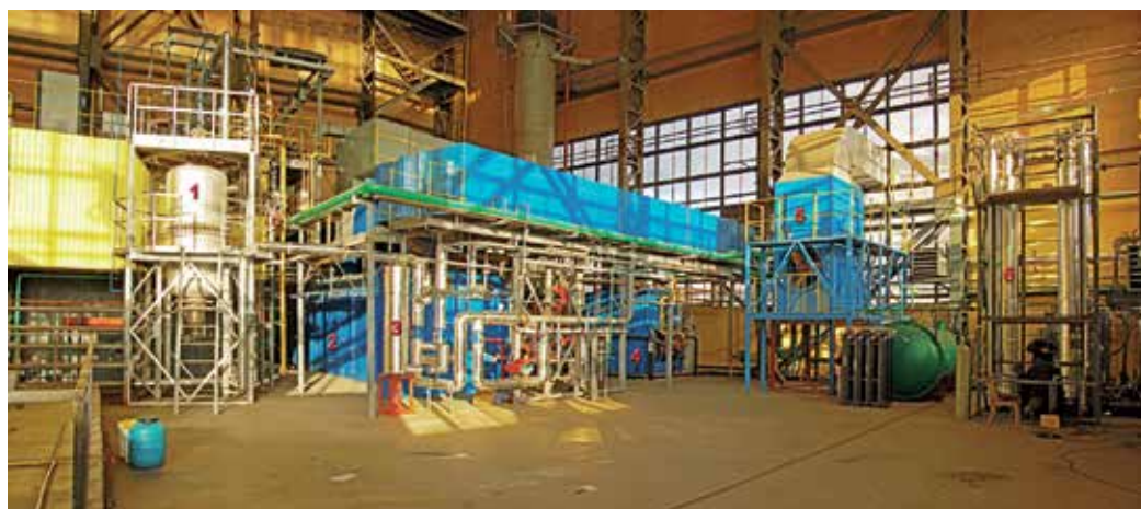
1 - The synthesis gas generator by partial gas oxidation with syngas cooler, 2 – gas turbine, 3- soot filter, 4 – water heating boiler, 5 – water cooling tower, 6 – block of methanol synthesis.
