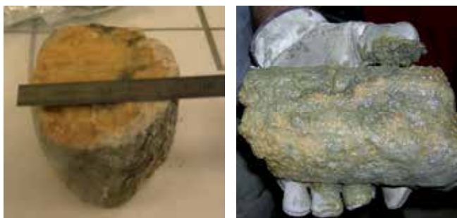
Fig. 2. Pictures of the recovered gas-hydrate specimens. The hydrates were massive and mixed with oily sediment.
