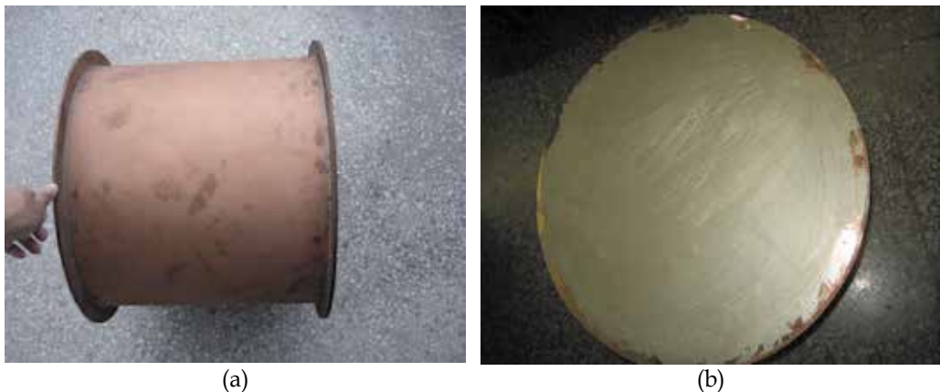
Fig. 11. (a) A resonating metal cavity following the theory in [19], (b) conducting ink on the wall
