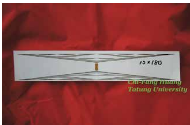
Fig. 5. A single RFID tag of UHF band made by offset printing technology
