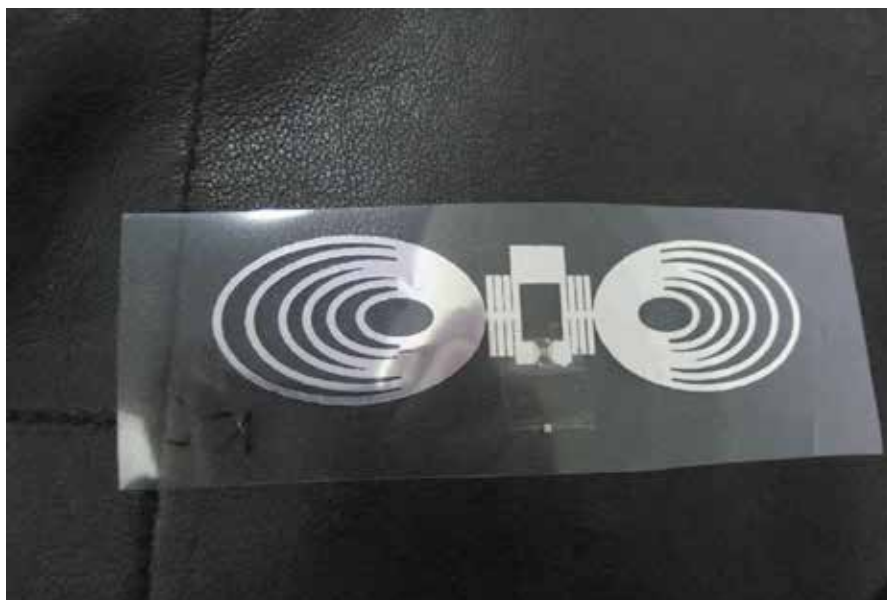
Fig. 14. A tag antenna using a company logo
