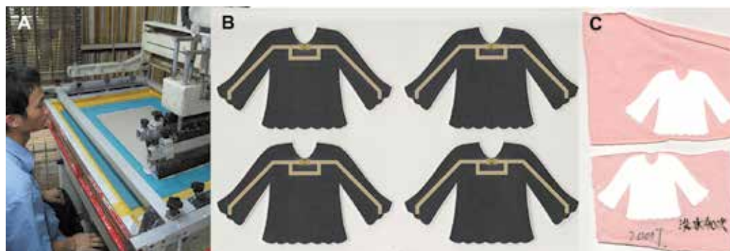
Fig. 2. Photographic images showing the RFID tag incorporated high reliability hot-press labels for garments. A) A worker is screen-printing the ultralow cost ECA based antenna in his work line in a company in Dongguan, China; B) A group of labels ready for heat-transfer printing; C) Samples cotton fabric pieces with the labels heat-transferred onto them. (Upper: before washes; bottom: after washing for forty cycles.) The RFID read range performance remained the same after the heat-transfer process and the subsequent washing cycles.
