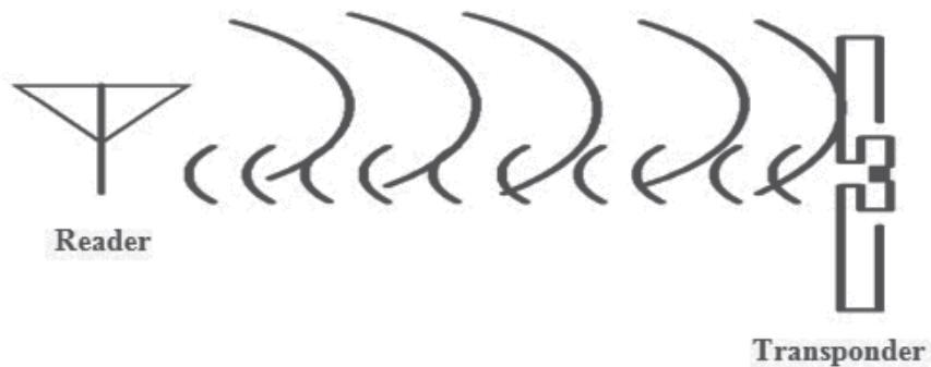
Fig. 6. Radiative coupling or far field detection of RFID reader
