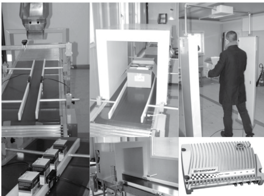
Fig. 2. Test environment composed of an items line (left), a cases line (middle), and a border gate (top right).
