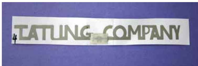
Fig. 13. A tag using the company brand being antenna's arm
