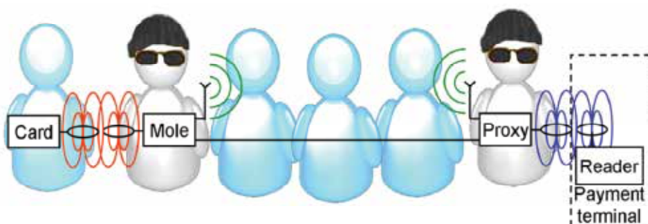
Fig. 12. Payment scenario: the relay attack setup
