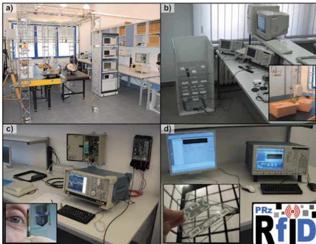
Fig. 9. RFID laboratory in the Rzeszów University of Technology: a) dynamic test stand, b) static test stand, c) example of long range read/write devices, d) example of measuring equipment
