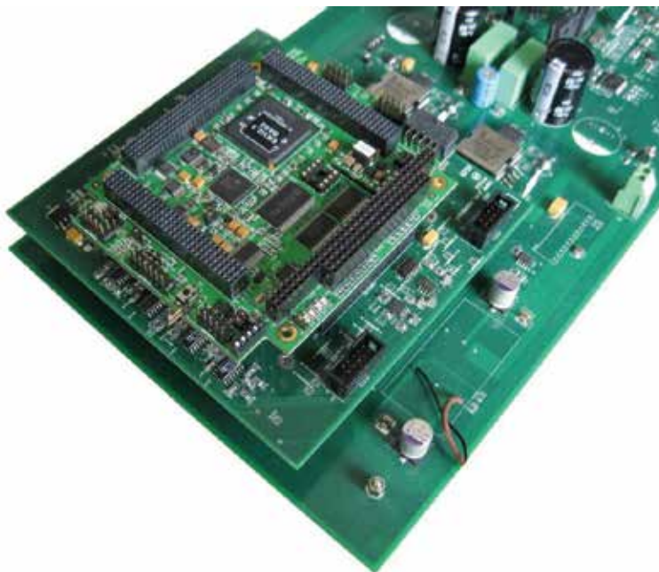
Fig. 11. The experimental set-up of the proposed FPGA controlled DC/DC step-up converter
