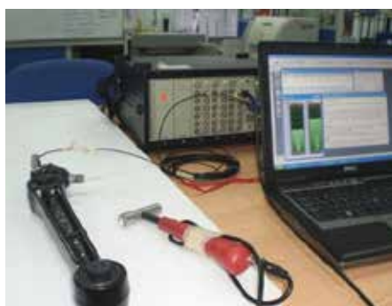
Fig. 6. The set up of data acquisition Portable Analyser Pulse to be used for normal mode analysis test
