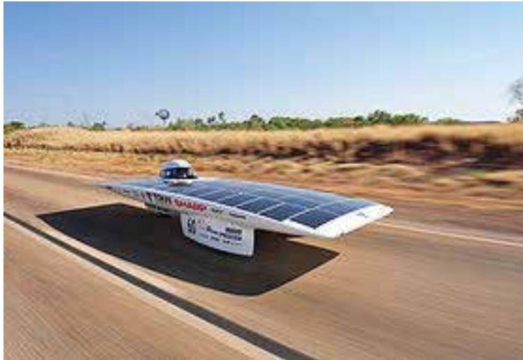
Fig. 5. WSC cars have large areas to place solar panels.
