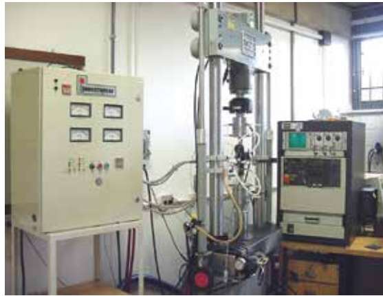
Fig. 6. Overall view of the testing apparatus, showing the induction furnace and the MTS 810 servo-hydraulic testing system.
