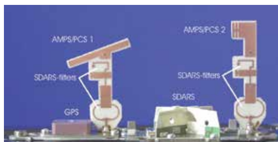
Fig. 10. Internals of a modern shark-fin antenna © IEEE with permission (J.F. Hopf et al., 2007)
