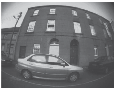
Fig. 6. Automotive fish-eye example illustrating the effects of fisheye distortion.
