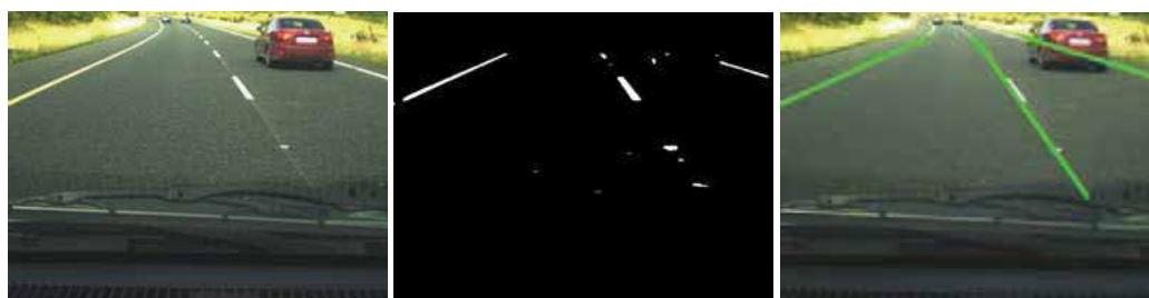
(a) Automotive image (b) Segmented roadmarkings (c) Detected lane boundaries
