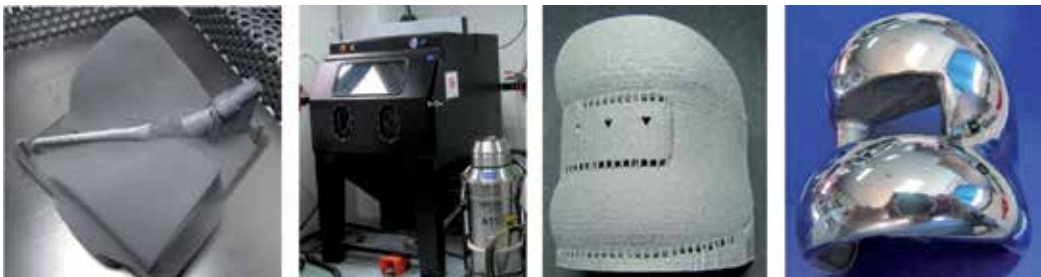
Fig. 13. Implant post-processing. From left to right: hip stem still involved by the powder bed; powder recovery system; knee implant as taken out from the machine and after support removal and hand polishing.
