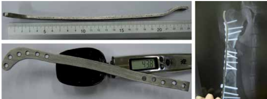
Fig. 23. Left: images showing size and weight of the customized plate. Right: post-surgery X-rays image of the plate (Courtesy of CIMA and FAUNA).
