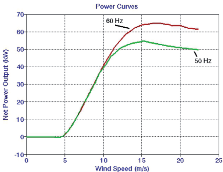
Fig. 6. Power curve for 15/50 Atlantic Oriental Corporation WTG [13].
