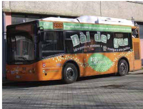
Fig. 15. Urban bus tested with HCNG blends (Genovese et al., 2011).
