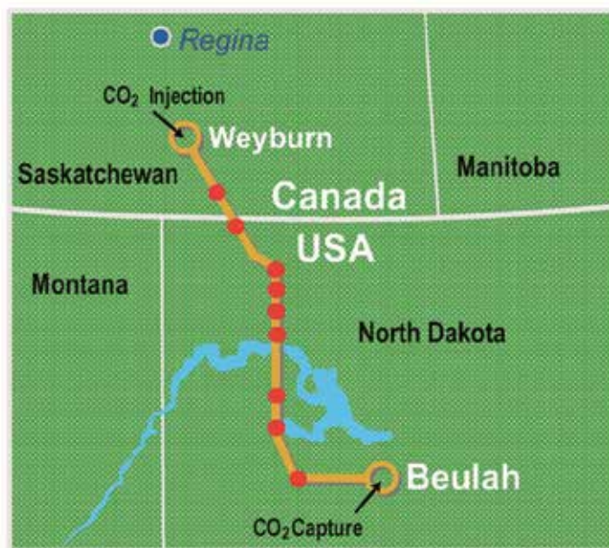
Fig. 11. Carbon pipeline linking Beulah and Weyburn – Source: Cenovus Energy (2011)
