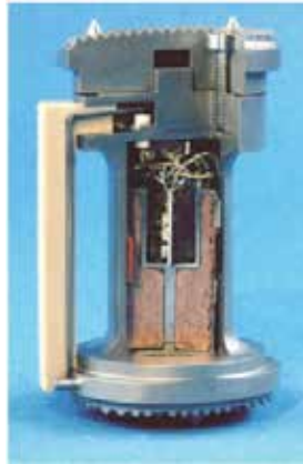
Fig. 25. Wireless load measuring system for vertebral body replacement (Rohlmann et al., 2007)
