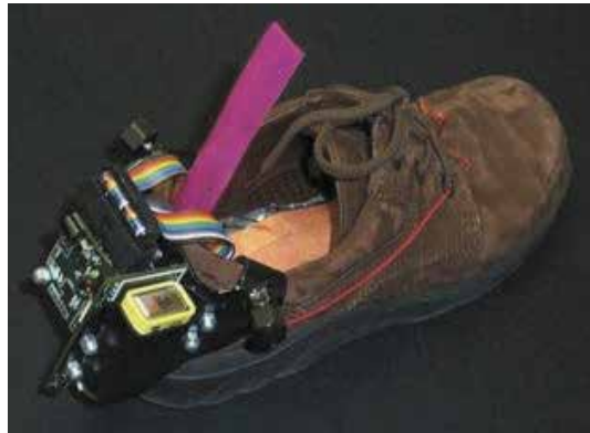
Fig. 23. Wireless gait analysis system (Morris & Paradiso, 2002).
