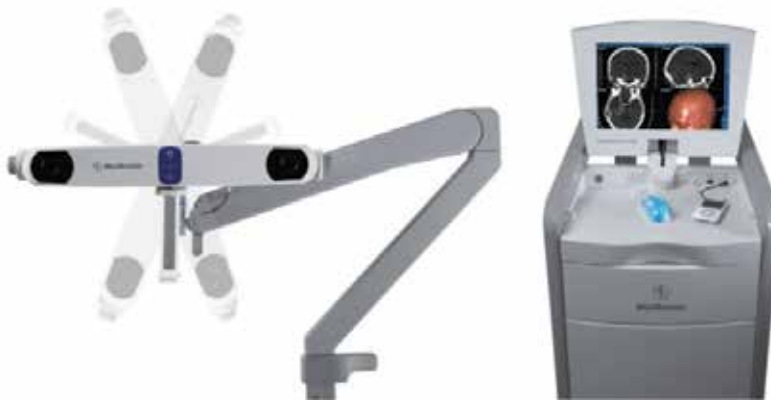
Fig. 18. Optical tracking devices for surgical navigation (Metronics).
