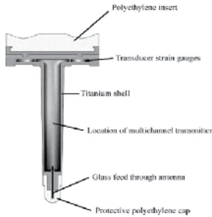
Fig. 26. Telemetry stress measuring knee implants (D'Lima et al., 2005).
