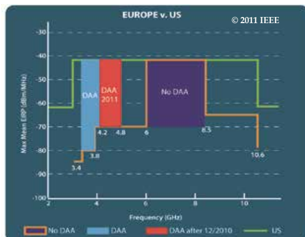
Fig. 4. Comparison of allocated UWB bands between 3-11 GHz in the U.S. versus Europe (Mahfouz & Kuhn, 2011).
