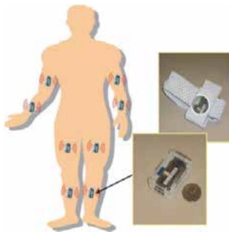
Fig. 22. A network of wireless sensing nodes consists of accelerometers (Patel, et al., 2009).
