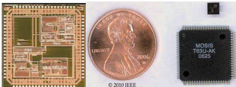
Fig. 55. ASIC designed for microcantilever readout (Left: ASIC footprint, Right: ASIC with testing package) (Qu et al., 2010)
