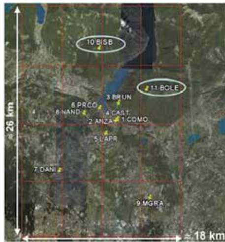
Fig. 3. Geographic distribution of the MisT network. The two “mountainous” GPS receivers are highlighted. The final volume discretization is also superimposed.
