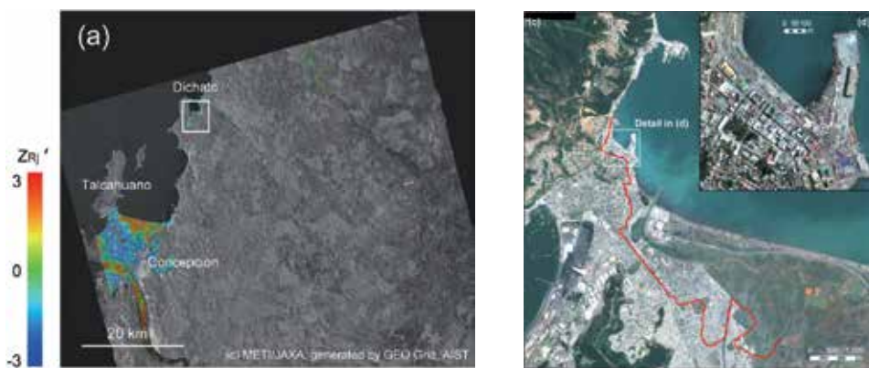
Fig. 14(a). Distribution of Z_{R2} obtained by ALSAR images in Talcahuano and optical images
