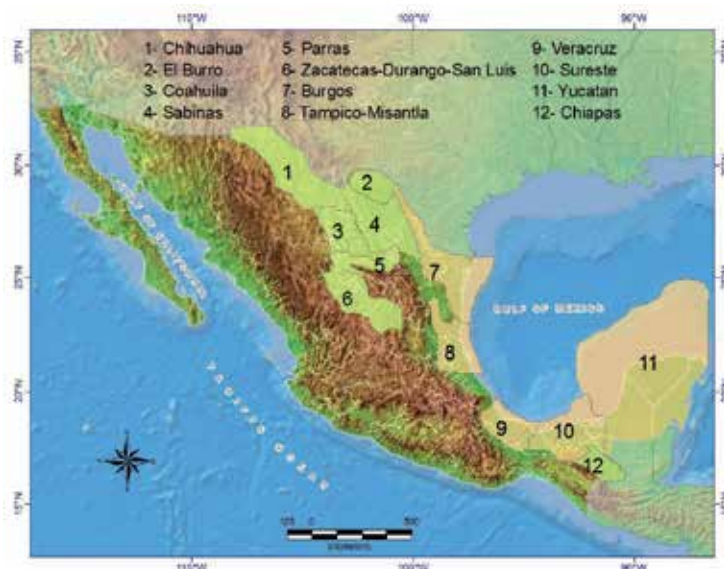
Fig. 4. Mexican geological provinces identified according to their underground potential for CO 2 storage.
