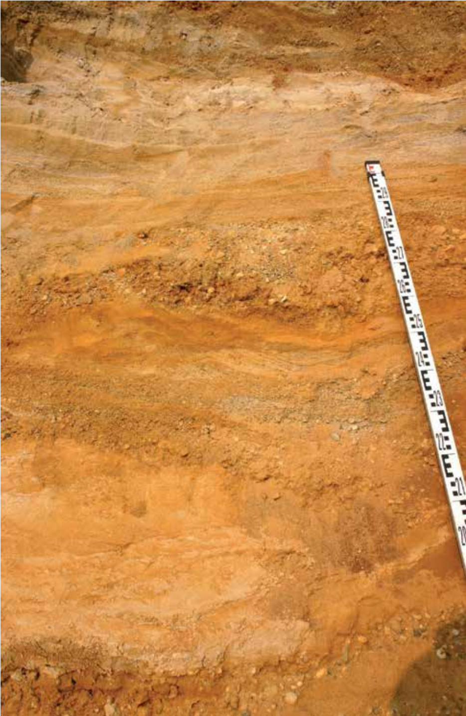
Fig. 15. Gravel-clay-sand fluvio-glacial deposits. Northwestern glaciation unit, mining open cast on the right bank of the Umbella River.
