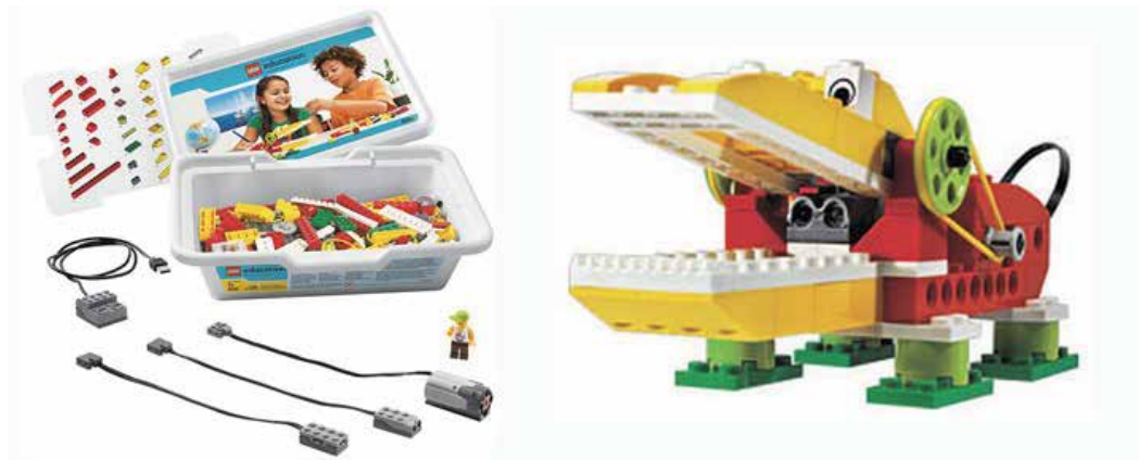
Fig. 6. Lego WeDo parts and a robot
