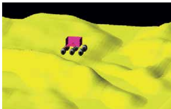
Fig. 12. Dynamics simulation of lunar rover with ADAMS
