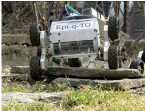
Fig. 17. Epi.q-2 traversing an obstacle, on uneven ground
