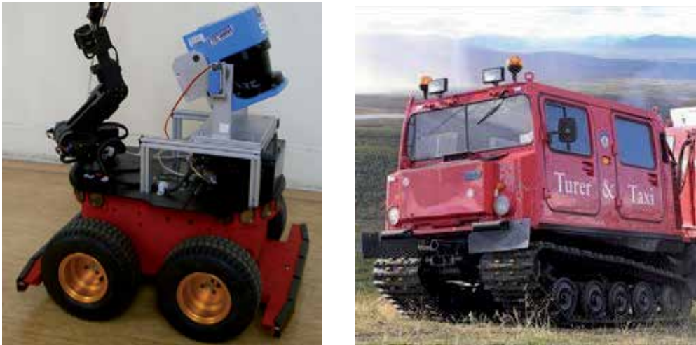
Fig. 1. Examples of skid-steered vehicles: (Left) Skid-steered wheeled vehicle, (Right) Skid-steered tracked vehicle
