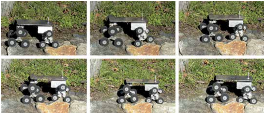
Fig. 12. Epi.q-1 in advancing mode, on uneven ground
