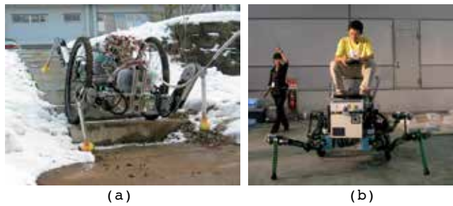
Fig. 1. A leg-wheel robot. (a)Chariot 3. (b)Chari-Bee is a demonstration robot of Aichi EXPO, 2005.
