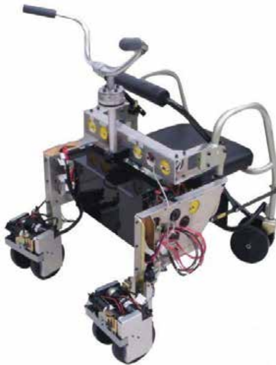
Fig. 1. The omnidirectional mobile robot in developing for the elderly's walking support, the disabled's walking rehabilitation, and the caregiver's power assistance
