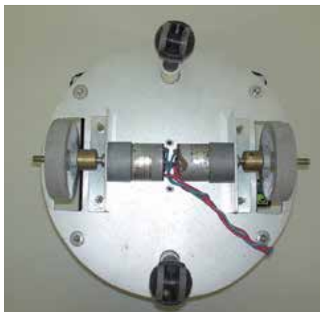
Fig. 11. The lower part of the Emmy II robot
