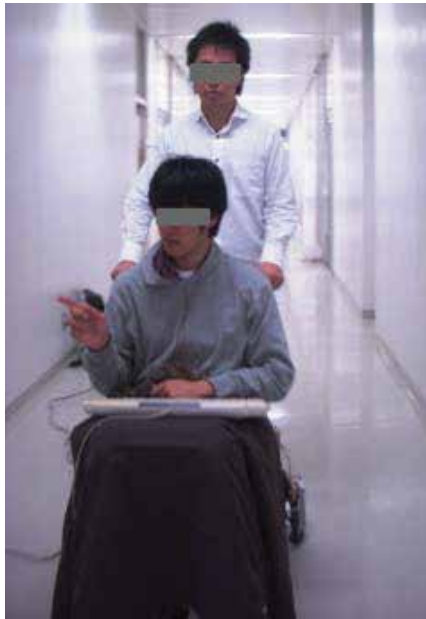
Fig. 7. A user pushes the robot while a person sitting in the seat.
