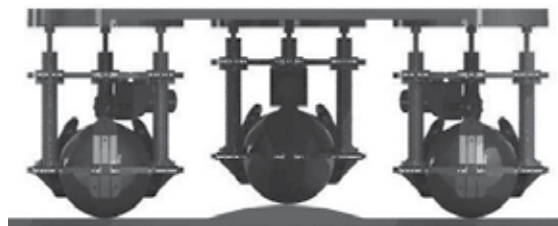
Fig. 5. Wheels adjustment with obstacle owing to proper action of suspension system.
