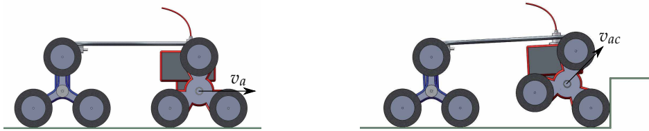
Fig. 6. Driving unit linear velocity during advancing mode, on the left, and automatic climbing mode, on the right
