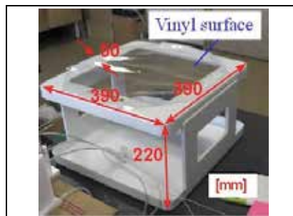
Fig. 6. Laparoscope operation simulation unit
