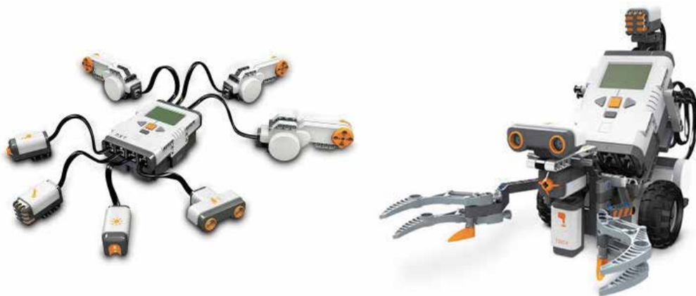
Fig. 2. Lego Mindstorms NXT Controller with sensors and a sample mobile robot
