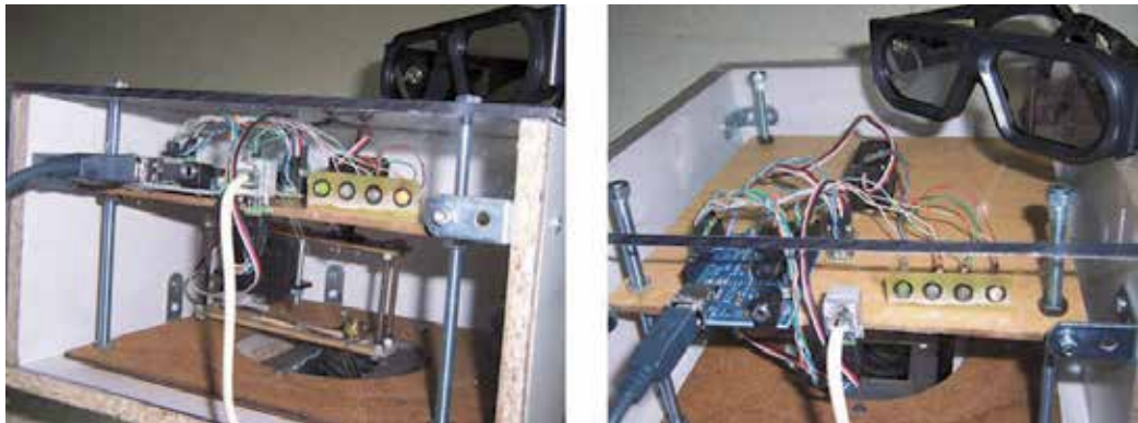
Fig. 11. Wheelchair joystick control prototype based on two servo motors, along with an adapted interface developed.
