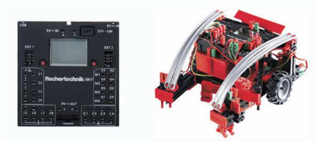
Fig. 3. Fischertechnik ROBO TX Controller and sample mobile robot
