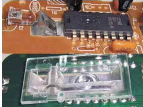
Fig. 4. Detail of the necessary components of the optical mouse for the adapted interface. The top of the image is the top view: LED, prism and integrated camera. The bottom of the image is the bottom view: prism and lens.
