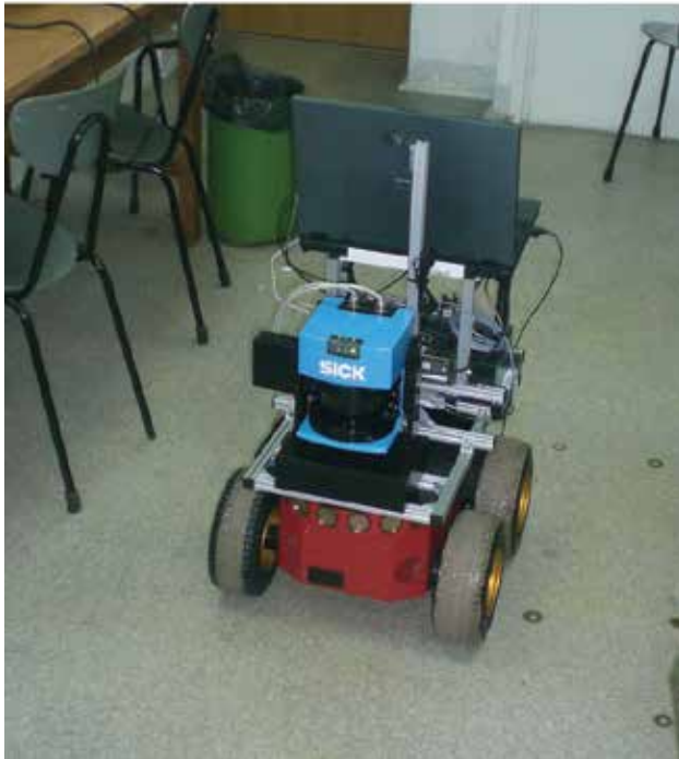
Fig. 10. Robot PIONEER 3AT equipped with 3DLSN sensor.
