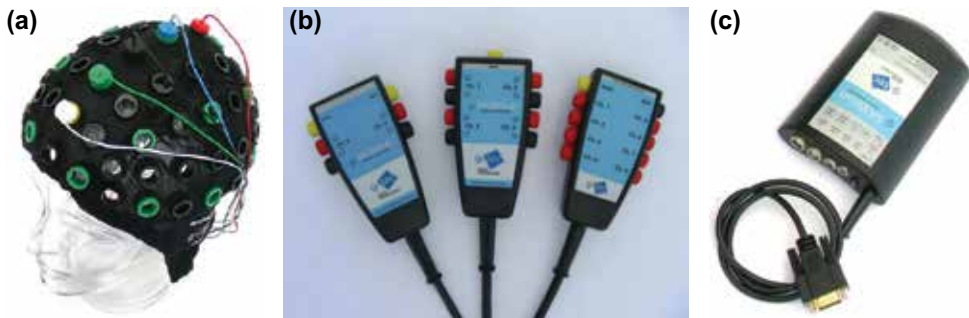
Fig. 7. EEG acquisition devices: (a) cap with electrodes, (b) connector and/or multiplexer, and (c) preamplifier.
