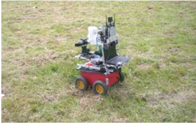
Fig. 8. Robot PIONEER 3AT equipped with Kinect sensor. Photo taken during Land Robot Trial CELROB 2011.
