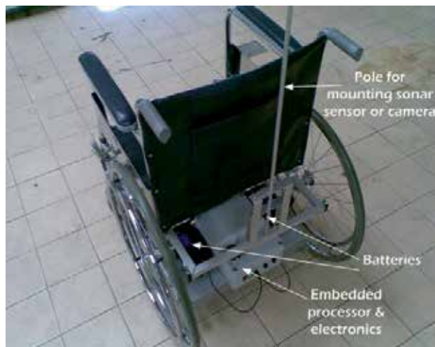
Fig. 1. The prototype of robotic wheelchair. The motorized wheels are under the add on unit
