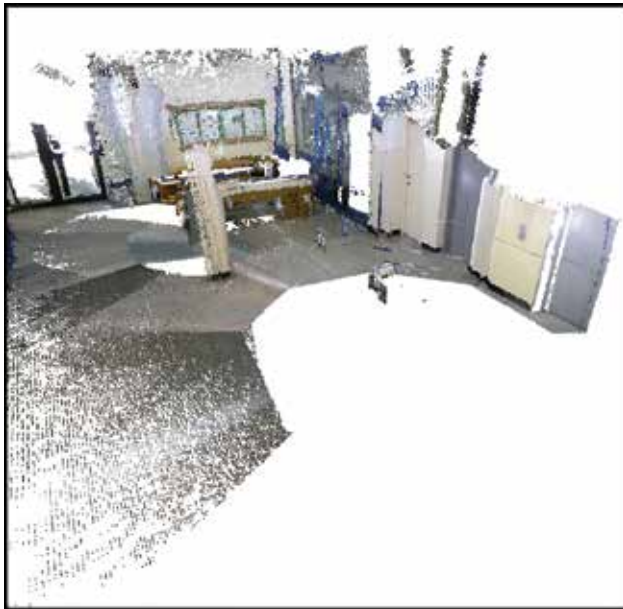
Fig. 9. Data registration using Kinect sensor. Result is satisfactory because of high resolution of Kinect sensor with acceptable level of noise.
