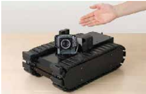
(a) Inspection robot YUKO-SHITA Sanyo.
