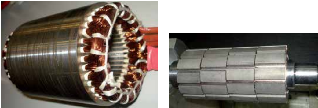
Fig. 5. Stator stack showing the motor laminations
