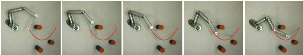
Fig. 15. Planar 4DOF manipulator tracking a path in an unstructured environment with three obstacles using velocity-based control (sampled every 1s)
