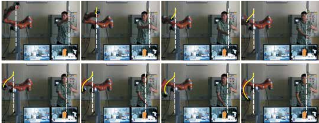
Fig. 16. A sequence of still photographs shows the movement of two Kuka LWR robots, while they successfully avoid each other. The desired movement for the robots is imitated in real time using the Microsoft Kinect sensor for the tracking.
