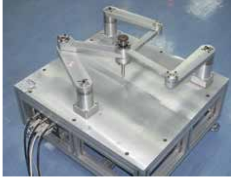
Fig. 2. The prototype of the 2-DOF parallel manipulator with redundant actuation
