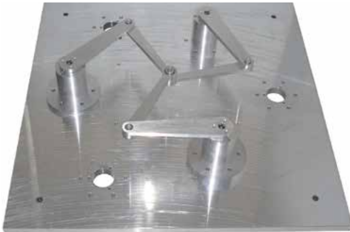
Fig. 1. Prototype of a planar 2RRR / RR RA-PKM.
