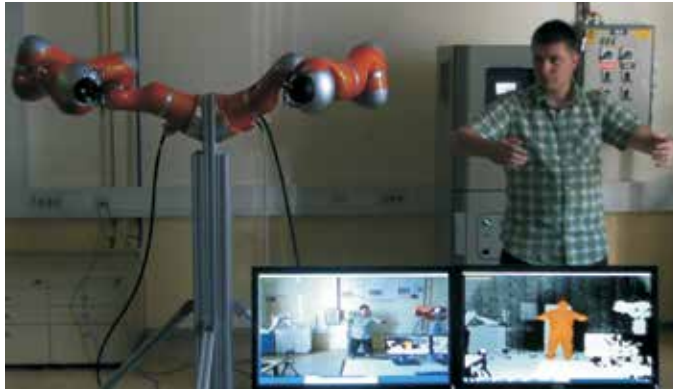
Fig. 14. Experimental setup with two KUKA LWR robots for bimanual movement imitation.
