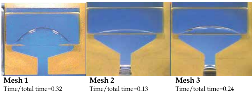
Fig. 5. Comparison of the effect of distributor geometry on the shape of the fluid front entering the mould for vertical mould orientation.
