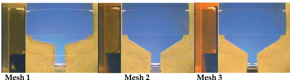
Fig. 7. Voids remain in the front upper and lower corners of each geometry for the vertical mould orientation. Each frame consists of two views of the mould (top view and side view). These voids can be seen more easily from the side view.
