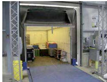
Fig. 4. Reader RFID for logistics purpose. Courtesy Deister Electronic.
