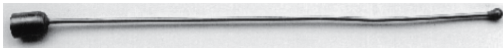
Fig. 3. Modified embryo transfer catheter. A machined brass zero-volume fitting was used to secure the catheter. From Wulster-Radcliffe et al., 1999.
