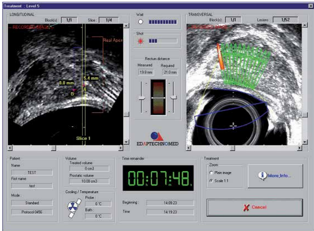
Fig. 4. On the screen, it is possible to follow the procedure and to change settings, such as ultrasound frequency and shot duration. Thus, a safe and optimal treatment can be performed.
