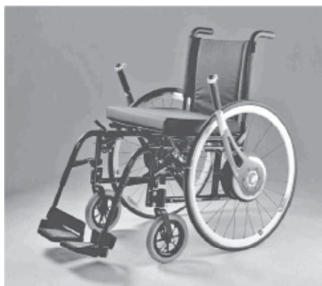
Fig. 6. Lever propulsion system (Requejo et al., 2008)
