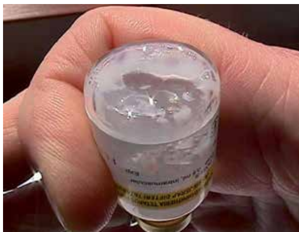
Fig. 10. Sub-zero temperature effect on DTP vaccine (after 10 minutes of vigorous shaking)
