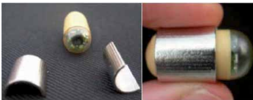
Fig. 4. Capsule with magnetic shield for controllable maneuvering (Capri et al. , 2011).
