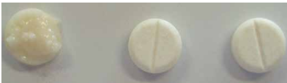
Fig. 2. Sodium valproate tablets after 21 days of storage at accelerated (40°C; 75% RH) (left), refrigerated (2–8°C) (middle) and controlled room temperature (25°C) (right) conditions.
