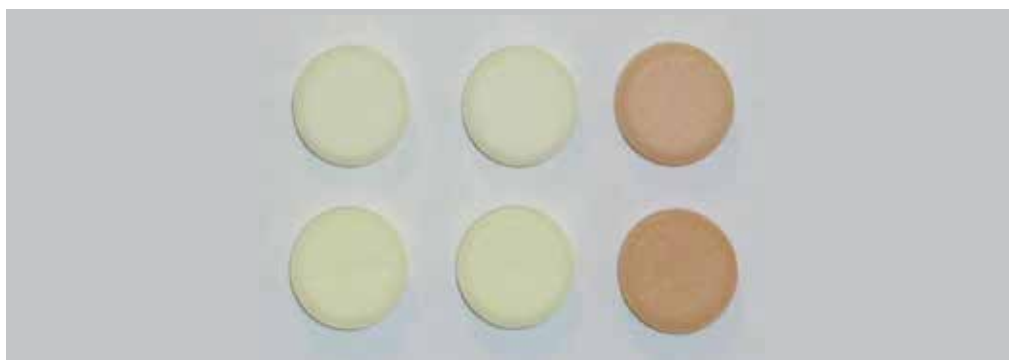
Fig. 6. Photographic comparison of the colour of clozapine tablets from left to right: control sample, sample stored in a DAA under simulated controlled room temperature conditions after 6 weeks, and a sample left out of the DAA packaging on the windowsill after 6 weeks (Clopine® above and Clozaril® below)
