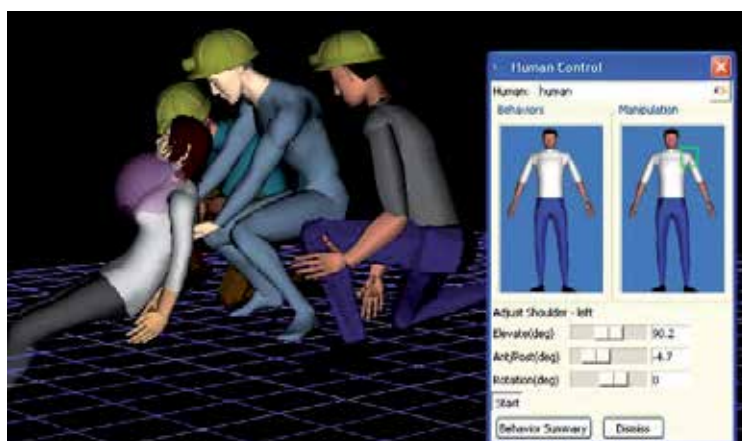
Fig. 37. The Human Control tab in JACK allows greater manipulation of the shoulder joint, pivotal in this task.
