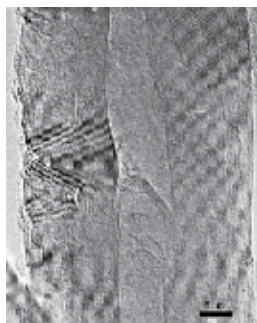
Fig. 4. HRTEM image of carbon nanotube prepared using catalyst with 3.5% iron (Wang et al., 2005a)
