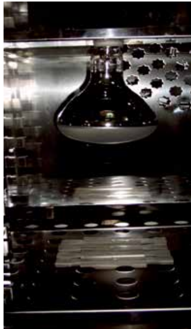
Fig. 1. Inside the climate chamber with 5 samples
