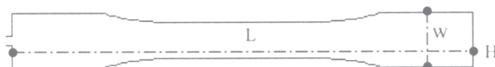
Fig. 1. Reference dimensions and their locations for shrinkage assessment of part length (L), part width (W) and part thickness (H)
