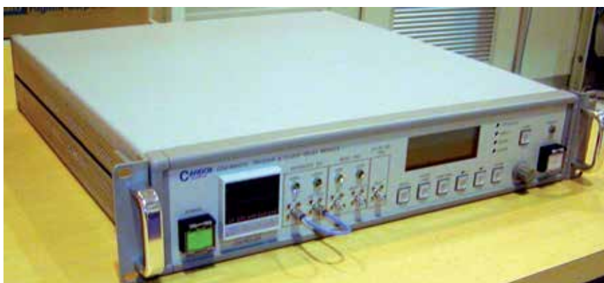
Fig. 6. High precision RF phase control circuit. The circuit provides a delayed RF signal from the output port with a precision of better than 3 ps (in rms) which is independent of the delay time.
