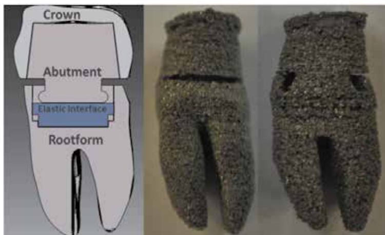
Fig. 9. Bio-adaptable dental implant with AAD (left), built by EBM ® (middle), cross-section of the build (right)
