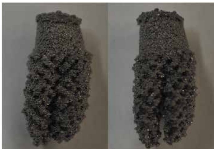
Fig. 10. Two bio-adaptable dental implants with porous rootform built by EBM ®
