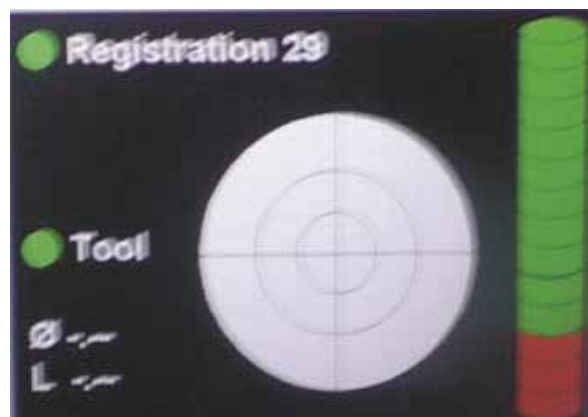
Fig. 24. Control panel of point of impact and drill angulation, the drill is represented as a sight with audible alarm.
