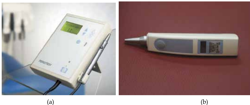
Fig. 2. Periotest® (Siemens AG, Bensheim, Germany) measures tooth mobility and implant stability by periotest value (PTV). (a) Periotest®, (b) Periotest®M.
