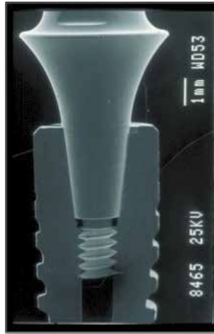
Fig. 6. Implant with a Morse taper implant-abutment connection and a microstructured surface treatment including the cervical collar and extending onto the implant shoulder.
