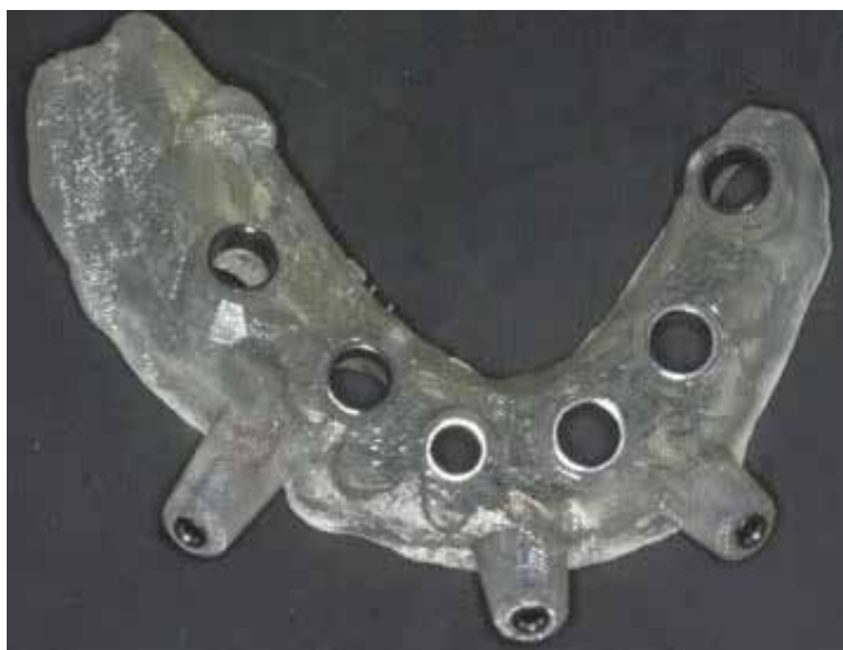
Fig. 17. Occlusal view of surgical guide: drilling orifices, stabilization cutter and implants direction.
