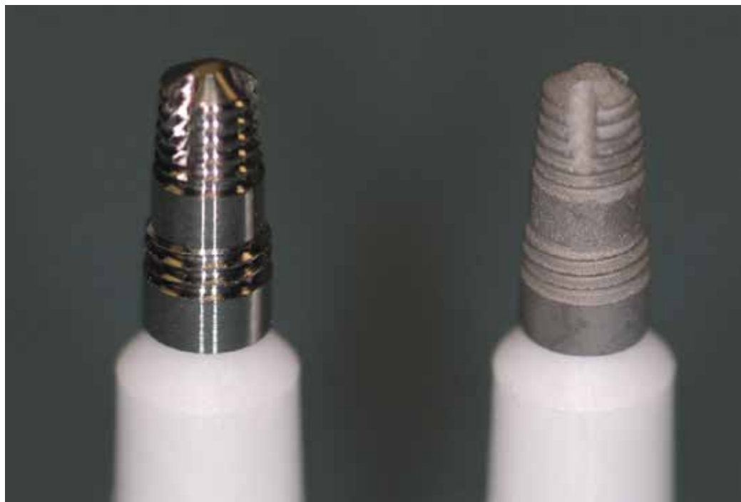
Fig. 3. The machined and nano etched implant surface
