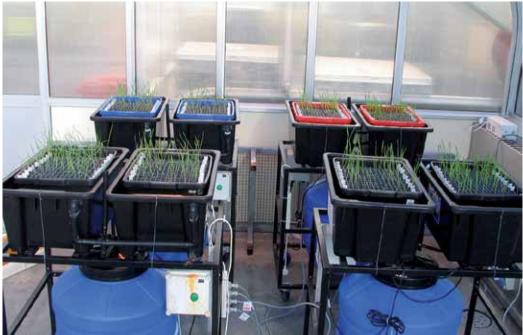
Fig. 1. A flood-drain 80 L supported hydroponics system in use at the Australian Centre for Plant Functional Genomics (ACPGF).
