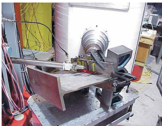
Fig. 9. Groove welded beam segment on neutron diffraction X-Y-Z translator table
