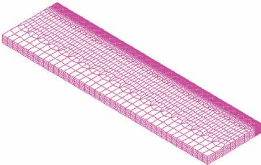
Fig. 27. Mesh of the plate being welded
