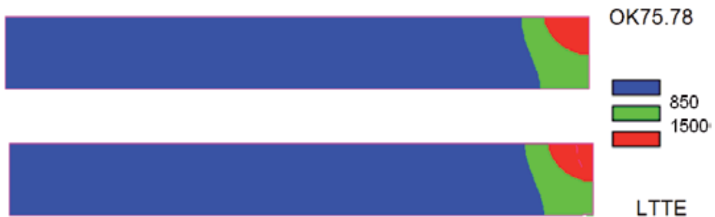
Fig. 28. Fusion zones produced for both cases.
