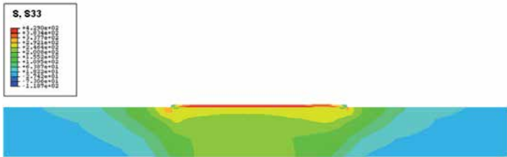
Fig. 17. Longitudinal stress (MPa); mixed hardening (Analysis B).
