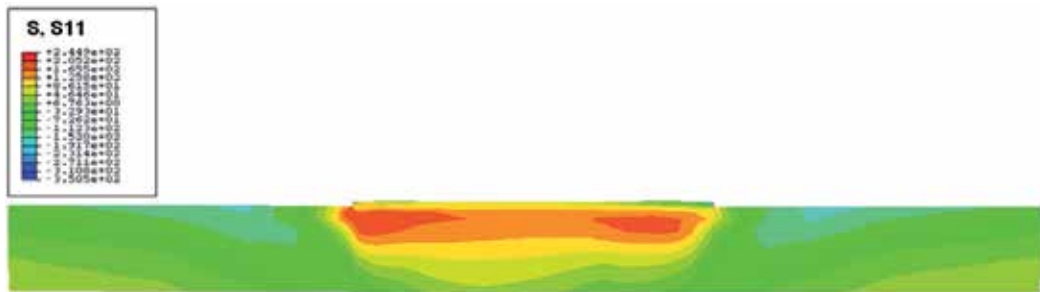
Fig. 18. Transverse Stress (MPa); mixed hardening (Analysis B).
