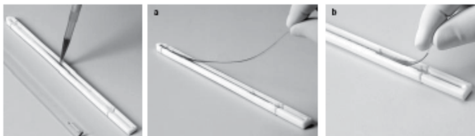
Fig. 4. The isoelectric focusing starts with application of the sample dissolved in rehydration buffer followed by inserting the IPG strip and covering with an oil layer to prevent evaporation. The assembly is then placed in a device that generates an electric gradient for focusing (ex, Ettan IPGphor) [from Amersham manual].
