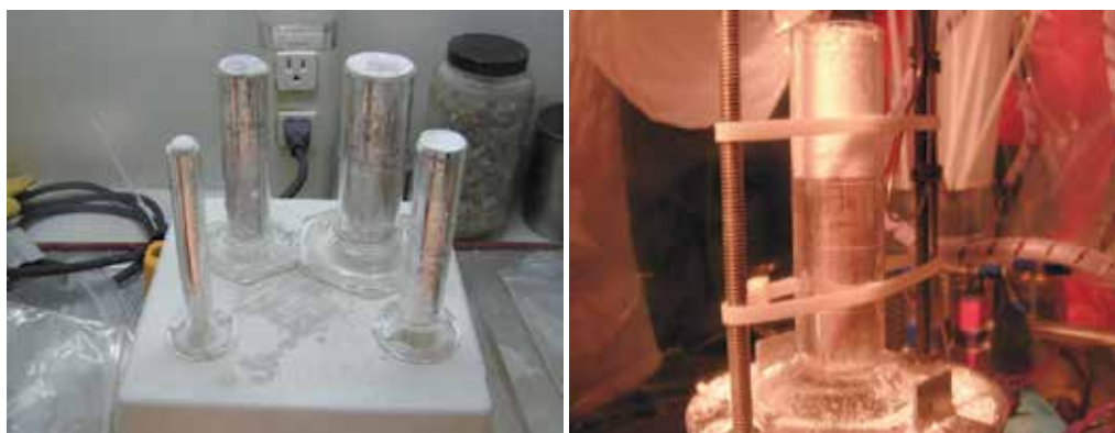
Fig. 5. Sodium samples before (left) and after (right) exposure to humidified \text{CO}_2 . In the figure on the right, the \text{NaHCO}_3 layer is visible as a white layer above darker gray sodium metal.
