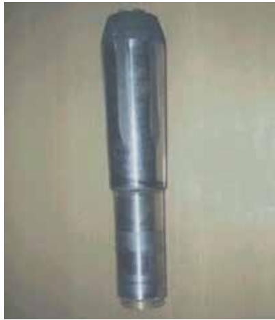
Fig. 7. Laboratory version of the flame jet pump system injection head (with permission of Professors Lazar and Sekula, Technical University of Košice, Slovak Republic)
