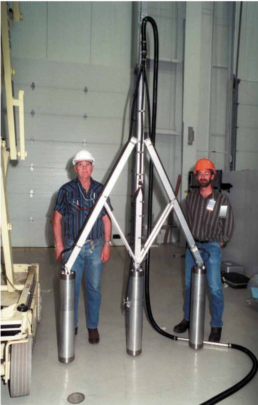
Fig. 3. Multi Detector Basin Scanning Array for INTEC-603.
