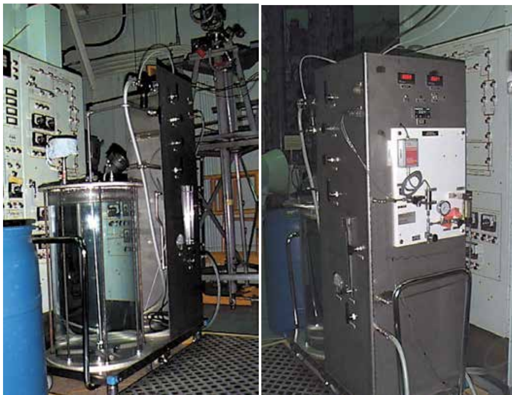
Fig. 7. Photos of the Humidification Cart's acrylic tank and instrumentation/valve panel.
