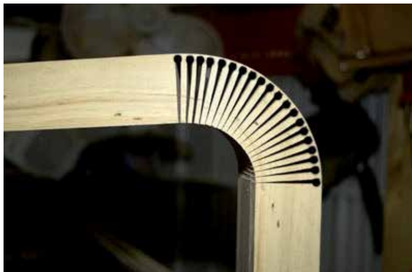
Fig. 6. A safe way to realize a serial incomplete wood cut for bending.
