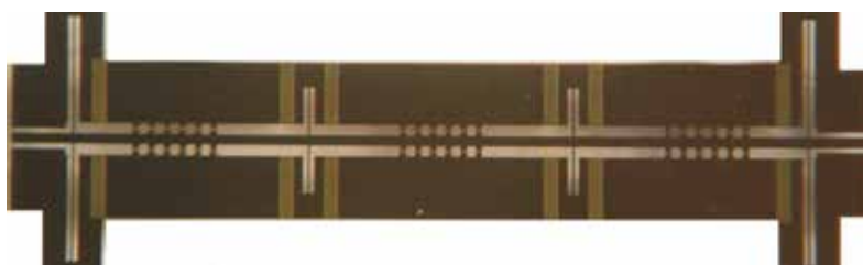
Fig. 21. A prototype of a 3-pole SWR filter with a total of 8 DC blocking capacitors
