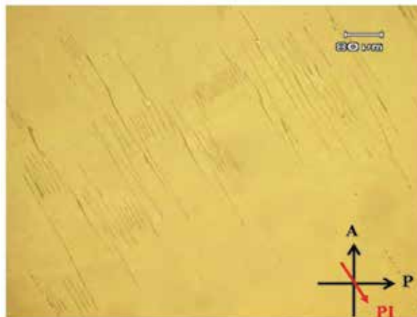
Fig. 4. The SSFLC texture of the FLC+1wt% BaTiO 3 at 30°C, under 200 times POM magnification. (The red arrow indicates the PI alignment rubbing direction)
