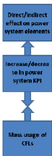
Fig. 7. Relation between using CFL (as a switch mode device) and the power system equipment.
