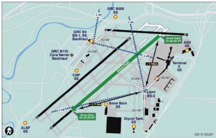
Fig. 12. AeroMACS mobility drive test on Runway 24L.
