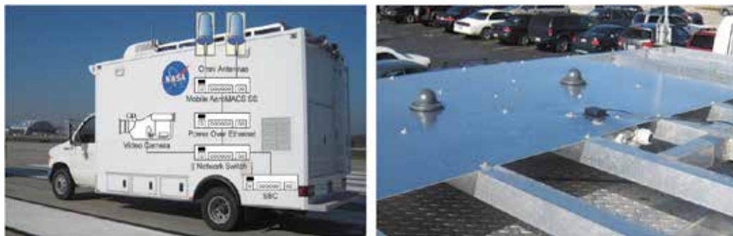
Fig. 11. AeroMACS mobile SS logical network superimposed on NASA Glenn Aeronautical Research Vehicle and roof-mounted omni-directional antennas for mobility testing.
