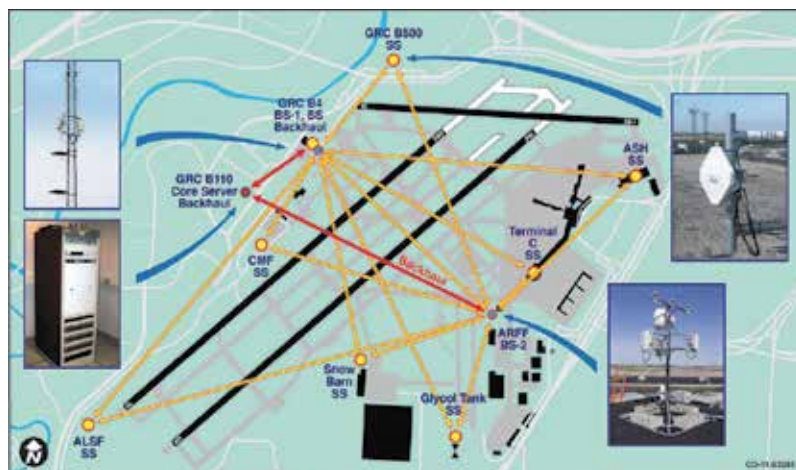
Fig. 9. NASA-CLE CNS Test Bed showing locations of the AeroMACS prototype base stations, fixed subscriber stations, microwave backhauls, and core server.
