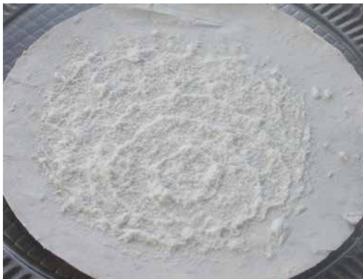
Fig. 6. Oscillating character in the filtering and washing process of the doped calcium carbonate-phosphate precipitation
