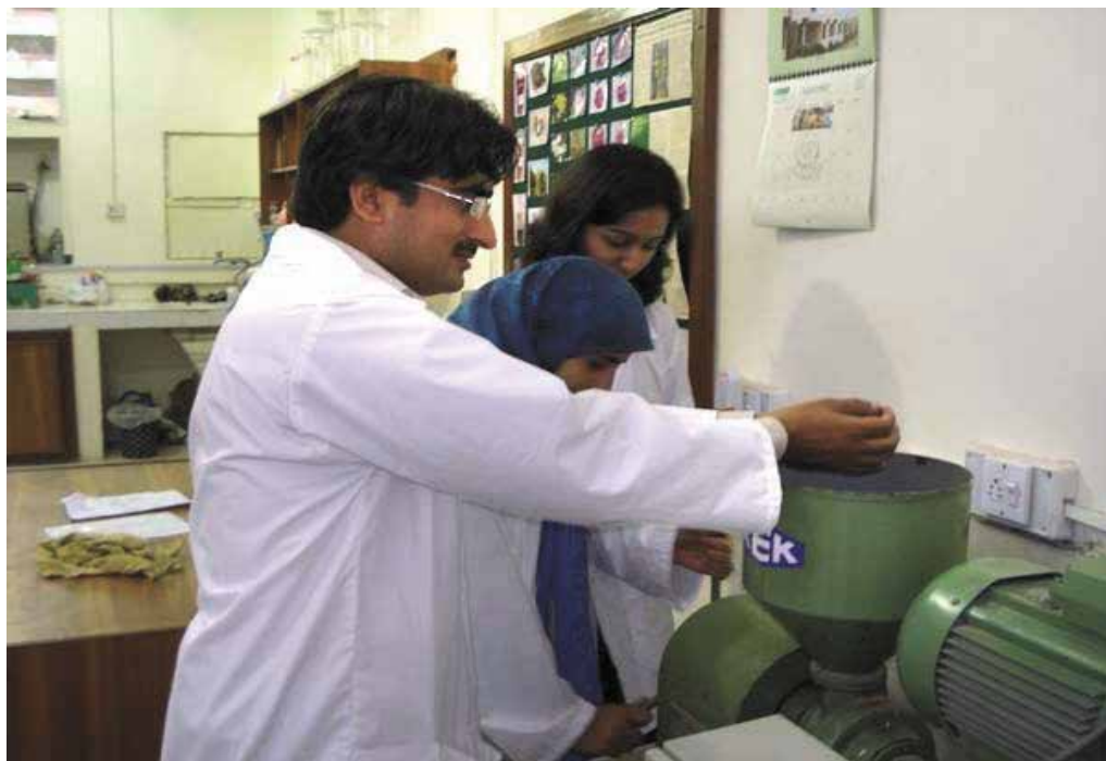
Plate 1. Extraction of oil by electric oil expeller
