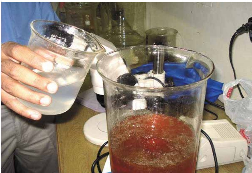
Plate 3. Mixing of sodium methoxide catalyst
