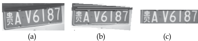
Fig. 2. Frame removal: (a) Original image; (b) The horizontal cut lines after corrected; (c) Frame removed
