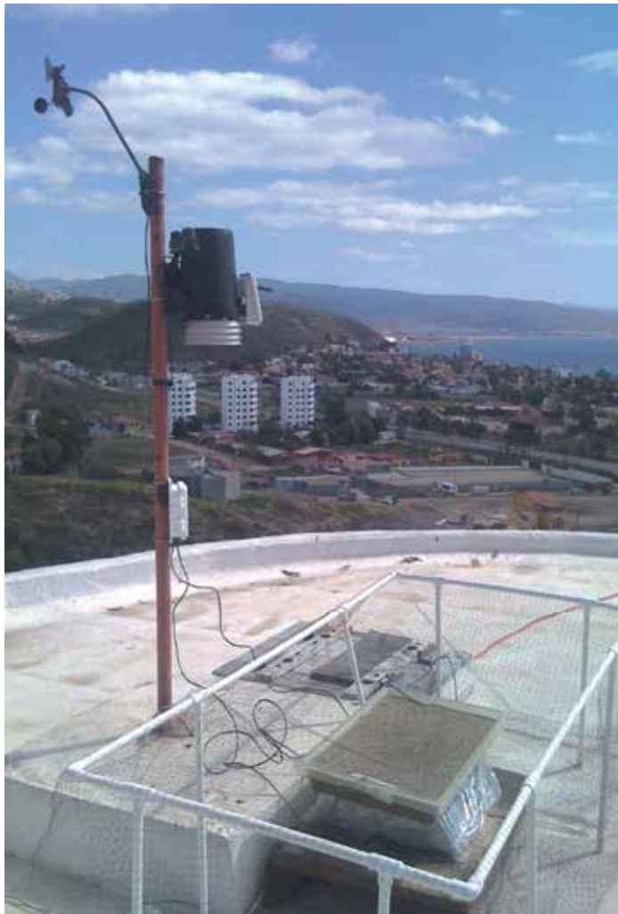
Fig. 1. The experimental setup: the meteorological station, the evaporative tray and the weighing scale used in the study.
