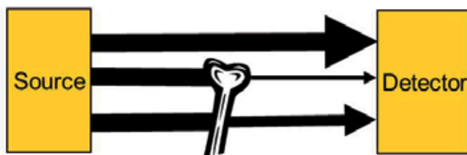
Fig. 1. Depiction of X-ray intensity attenuation as it passes through a tissue. X-ray attenuation is proportional to tissue mass.
