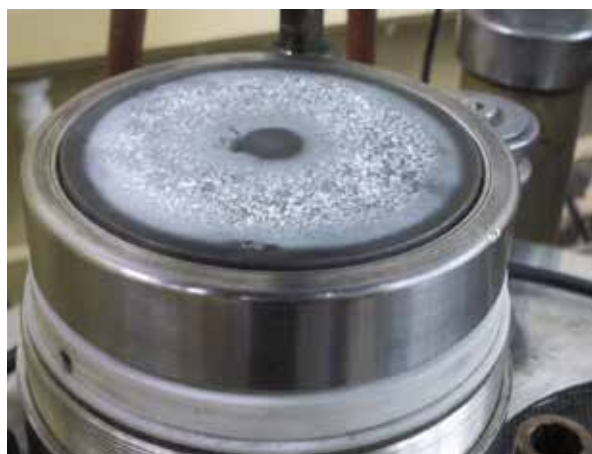
Fig. 2. The zinc target installed on the WMK-100 magnetron
