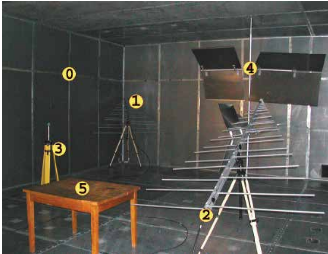
Fig. 30. Inner view of LASMEA MSRC ( 6.7 \times 8.4 \times 3.5 \text{ m}^3 ). Characteristics: (0) walls, (1) emitting and (2) receiving antennas, (3) field's probe, (4) mechanical stirrer, (5) working volume.
