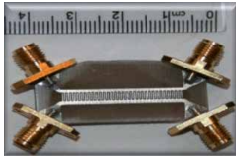
Fig. 21. Proposed forward symmetrical coupler which realized on FR-4 substrate ( \epsilon_r = 4.6 , h = 1.6 \text{ mm} ) (Keshavarz et al., 2010).
