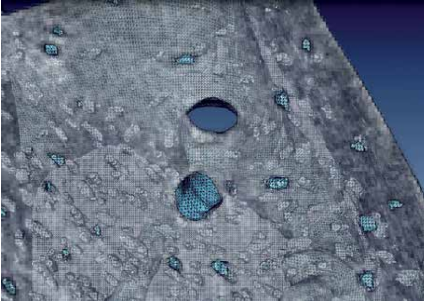
Fig. 14. Detail (through-view) of the FE-Mesh of the bone and osteocytes embedded in the bone matrix.
