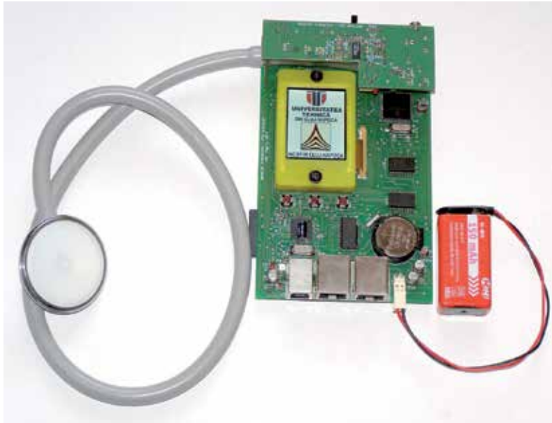
Fig. 27. The working prototype of the PCG signal analyser
