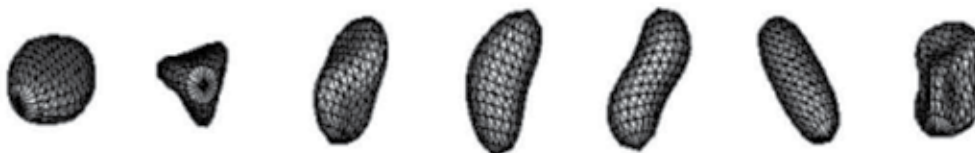
Fig. 2. Graphical representation of seven low frequencies vibration modes for surface model of ellipsoids [Syn and Prager, 1994]
