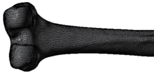
Fig. 27. Triangle surface grid of femur bone.
