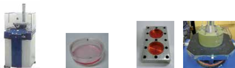
(b) Impact machine (c) Cultured dish and culture solution (d) Specimen container (e) Impact table
