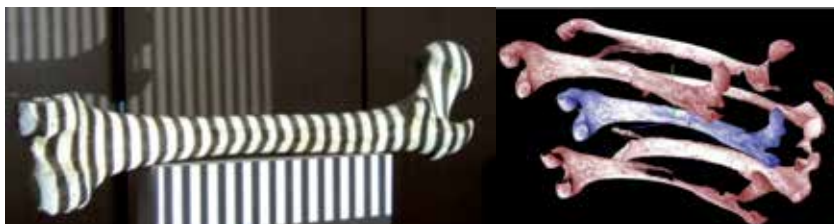
Fig. 23. Data acquisition process on 3D structural light scanner and set of points clouds.
