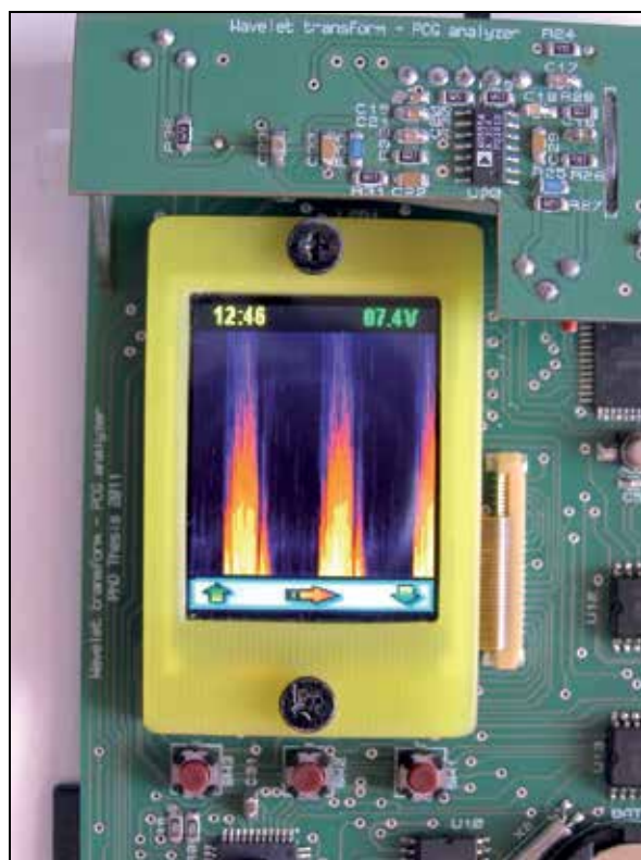
Fig. 28. Time-frequency scalogram of the „Aortic stenosis“ pathology
