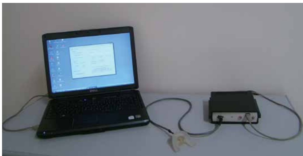
Fig. 3. Portable device for measuring the force of the tongue: Portable FORLING.
