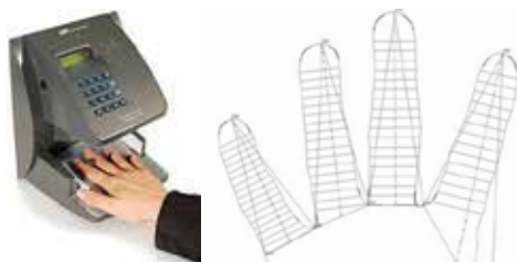
Fig. 15. Hand biometrics (from left): 2D biometric hand reader, segmentation of length and weight of the hand fingers features [Sanchez-Reillo R. at al., 2000].
