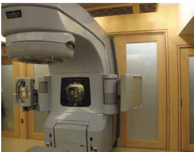
Fig. 10. Linear Accelerator with kV imaging arms attached. VARIAN 23 iX with OBI (On Board Imager).
