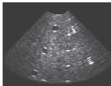
(d) The corrected image using the phase-aberration profiles derived using the steering angle-based sub-array method after manually adjusting ambiguity profiles.
